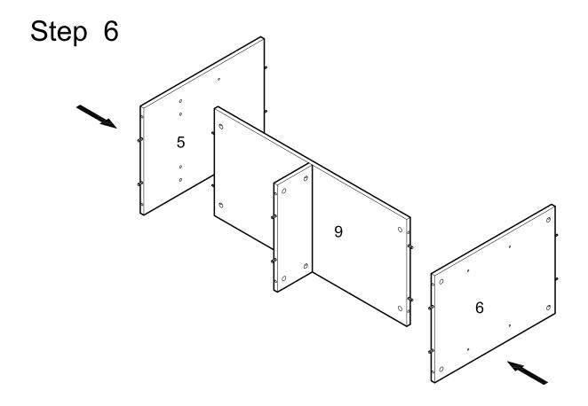
Attach panels (5,6) to panel (9) using cam bolts and dowels as guides.
